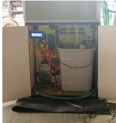
Figure 39. Overall view of working Ebb and Flow Hydroponics System
