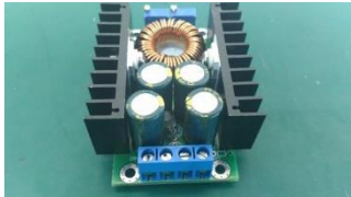
Figure 7: 300 watts Buck converter dc to dc
